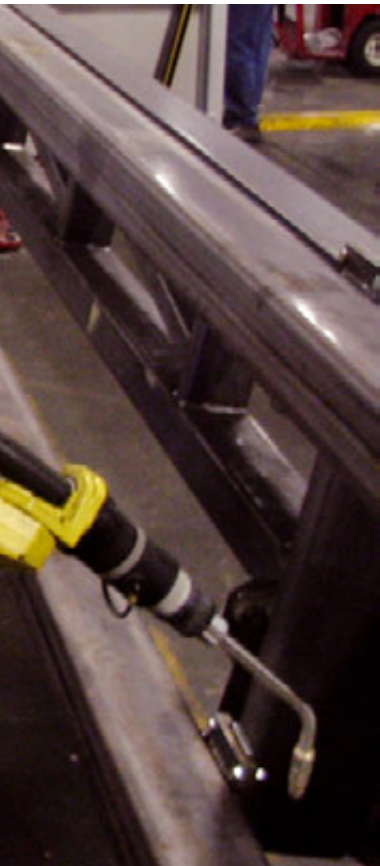
Automated welding of steel girders – a typical application in the transportation industry.
