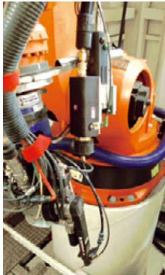
Laser soldering head AL01 with Master Feeder in frame size 1 and special liner.
