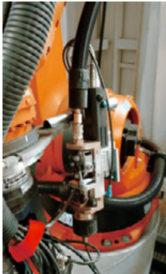
Four-roller drive with integrated wire speed indicator in detail.
