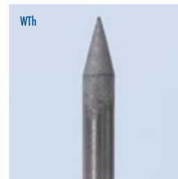
Much less consumed after 150 ignitions - E3 ® vs. WTh 20 electrode tips.
